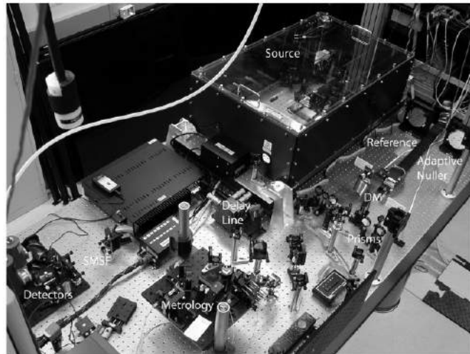
Adaptive Nuller Testbed at JPL (~2008)
